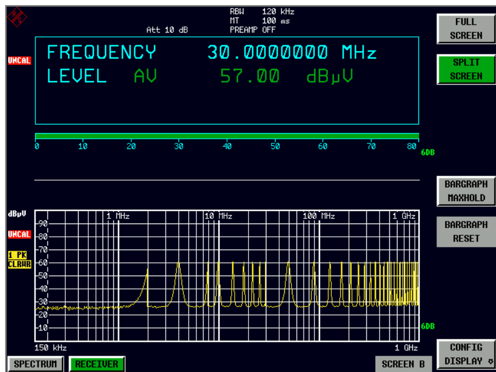
Fig. 4.16 Typical split-screen display
